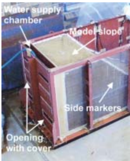
Fig. 5 Photo of the experimental soil box
