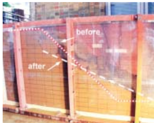
Fig. 11 Photo showing the model slope after the test (Case 6)
