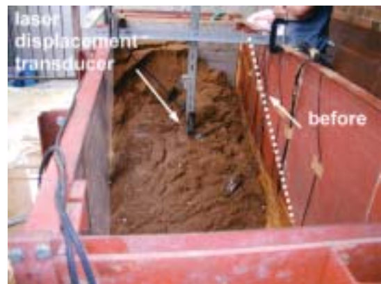
Fig. 13 Photo showing the model slope after the test (Case 7)
