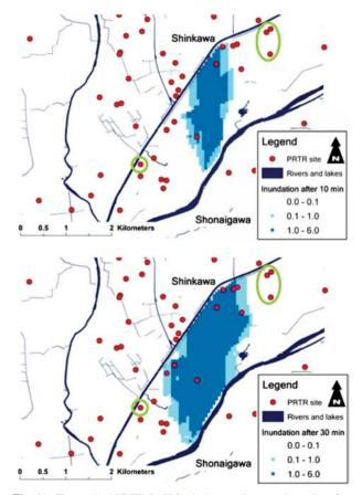
Fig. 4 The marked PRTR-facilities had more than one-hour time for preparation and were inundated with less than one meter height. Compare with Fig. 1.
