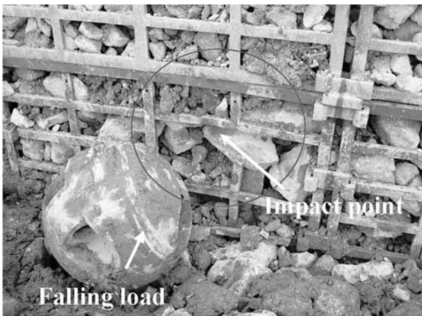
Photo 7 Panel after collision with 1.67 kN
