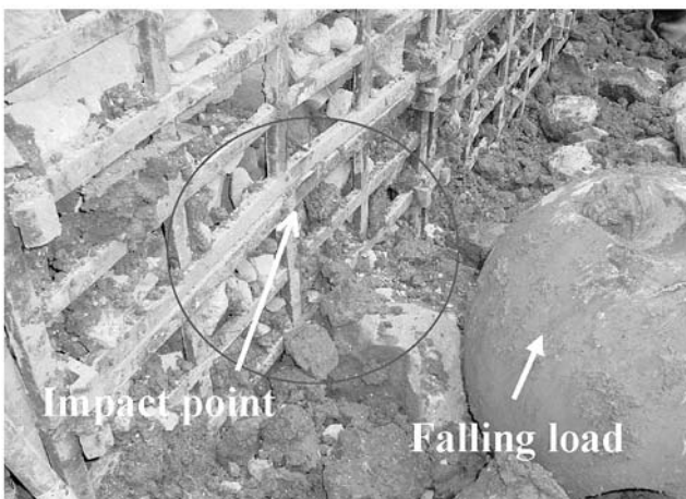
Photo 8 Panel after collision with 5.00 kN
