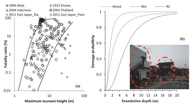
Figure 10. (a) Comparison between the tsunami fatality ratio from this event and from other historical events in Japan and the 2004 Indian Ocean tsunami and (b) damaged condition of an RC building, two-story wooden house and one-story wooden house under the same inundation depth of 4 m in Ishinomaki (26/4/2011)
